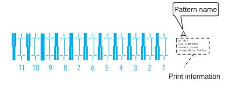
• For the Adjust print pattern, the same patterns will be printed repeatedly on both sides and center of the media.
