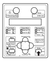
• An adjust print pattern is printed. For Adjust print pattern printing, 6 adjust print patterns (A to F) are printed. Enter the adjusted values.
