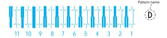
• For the rough adjustment pattern, the same patterns will be printed on both sides and center of the media.
