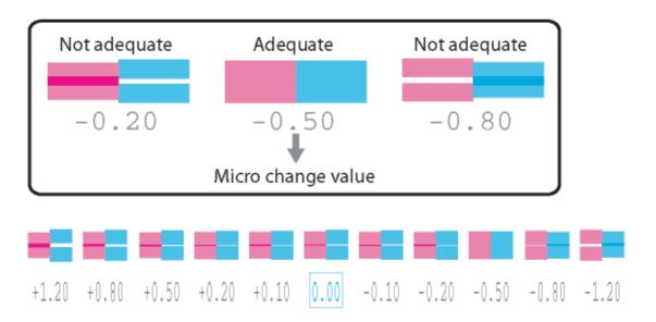
• After the micro adjustment printing is completed, "Micro Change: 0.00%" is displayed on operation panel.
