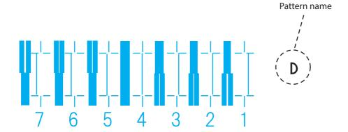
• For the micro adjustment pattern, the same patterns will be printed on both sides and center of the media.
