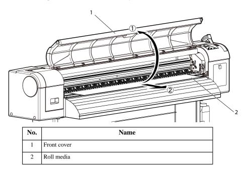
5. Wind back the roll media with the scroller to remove a media warp or skew.
